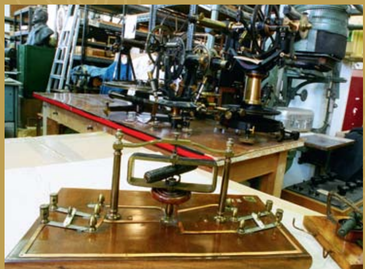
Ányos Jedlik's lightning-magnetic self-rotor (electric motor) Photos: MTI
